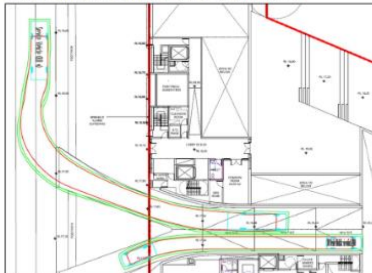
Figure 3 Sweep Path Assessment - 99 th Percentile Car Entry/ 8.8m Medium Rigid Vehicle Exit
